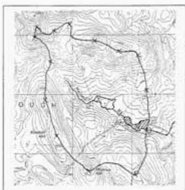
Figure E-5: Delineating a Watershed Boundary - Step 2
